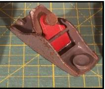
Finger plane can be used to fair in roof.
