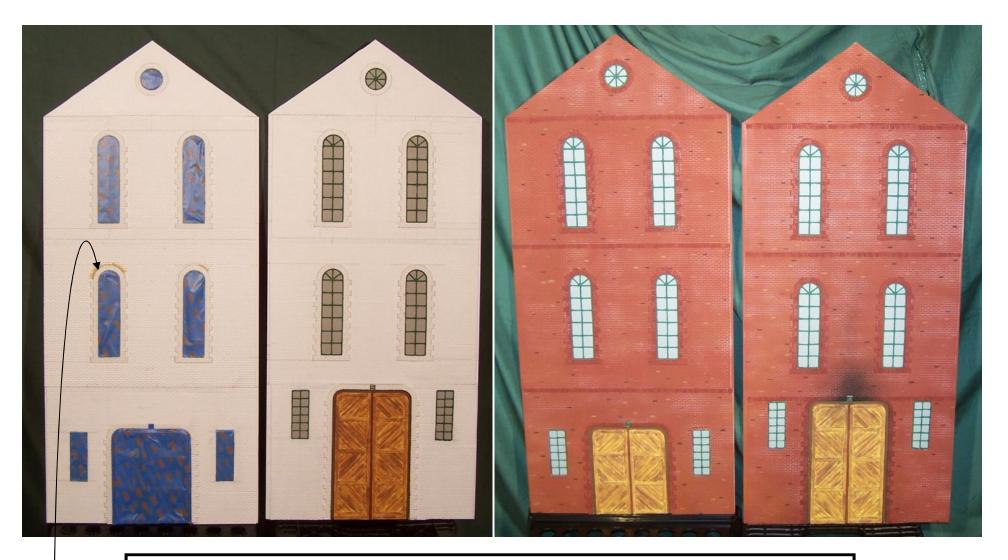
Build sides on a flat surface. Paint windows and doors first. Mask off. Paint brick in order shown on BoM. Note random brick coloring
